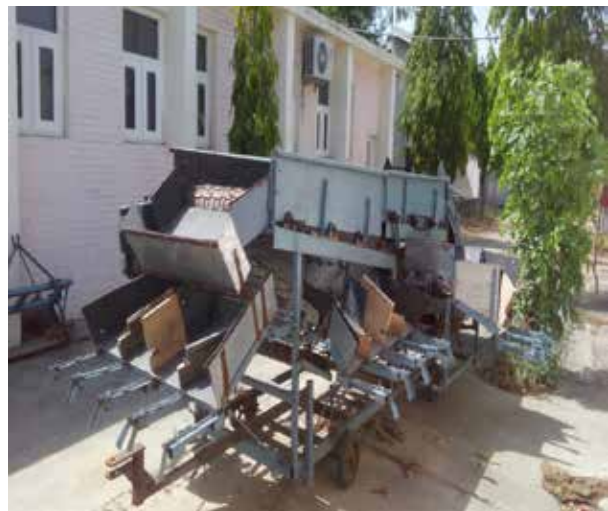
Fig. 1. Square wire mesh type of potato grader
