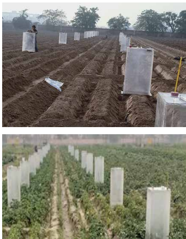
Figure-1-Collection of GHGs samples from field using the closed-chamber method.
