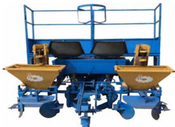
Fig. 9. ICAR-IISR sugarcane-cum-potato planter
