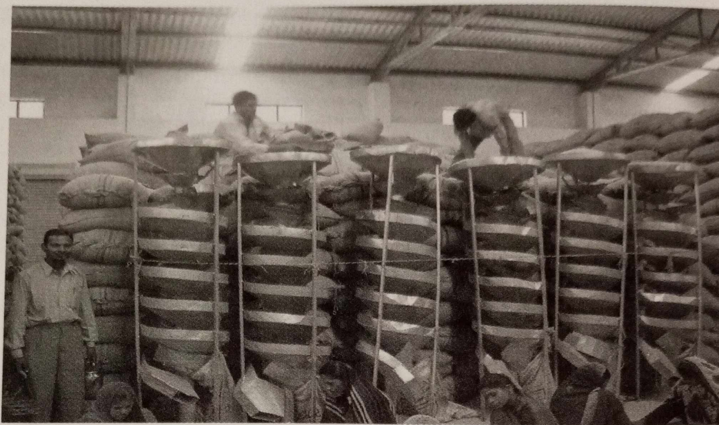
Fig. 1. Series of spiral separators being manually fed with soybean seeds
