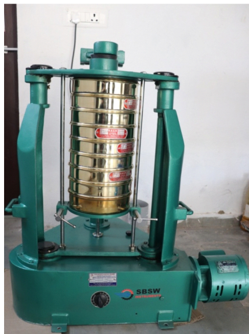
Figure 1. Sieve Shaker (Model No. SB5W)
