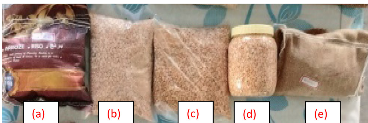
Fig.1. Pigeon pea dhal stored in different packaging materials (a) BoPP; (b) HDPE; (c) LDPE; (d) PET; and (e) Jute bag
