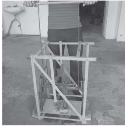
Fig. 10. Laboratory model rice transplanter during operation
