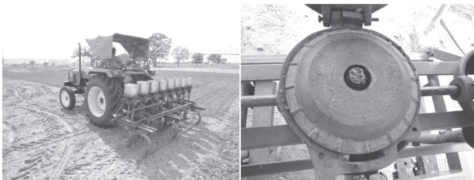
Fig.2. Nandyala planter with horizontal plate seed metering mechanism
