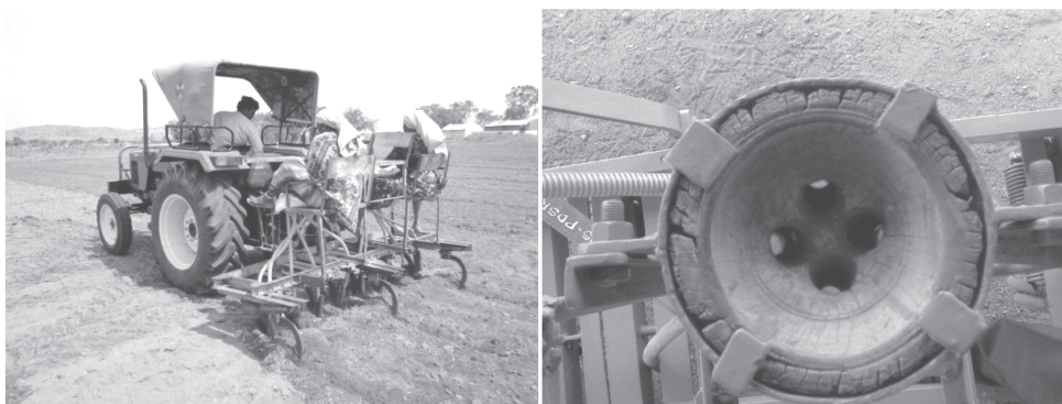
Fig. 5. Local seed drill with manual dropping seed metering mechanism
