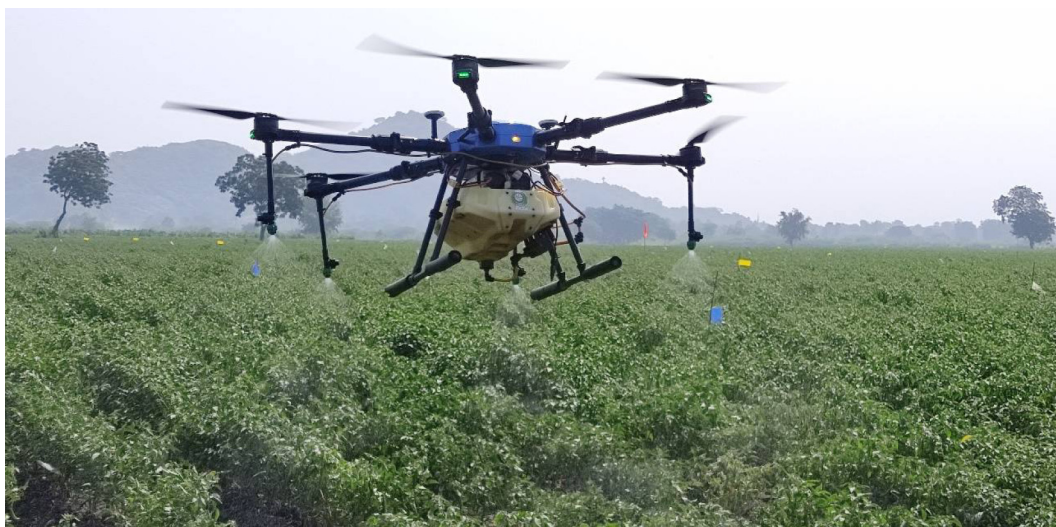
Figure 2. An UAV spraying of recommended chemicals for bio-efficacy and phytotoxicity studies
