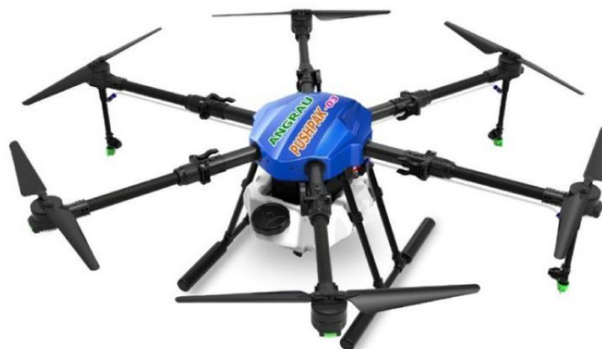
Figure 3. ANGRAU-PUSHPAK 01 - An UAV standardized for agricultural spraying
