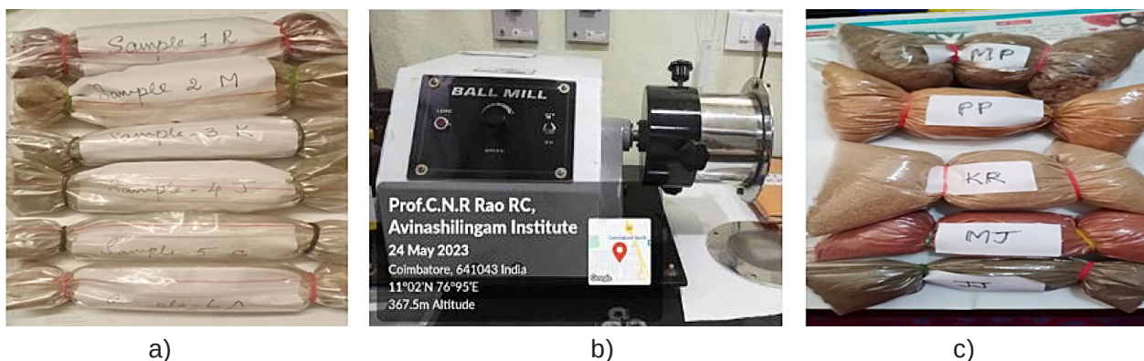
Fig. 2. a). Coarsely ground powders b). Ball mill c). Ball-milled powders.
