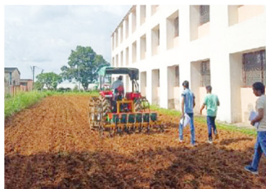
(b) Sowing and Fertilizer application with Tractor operated 6 row planter with fertilizer drill
