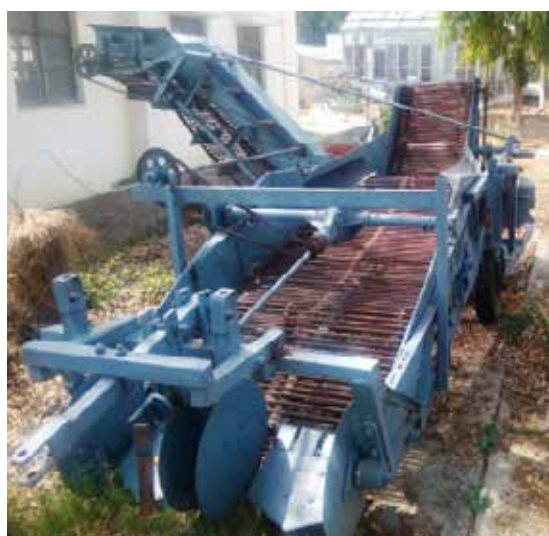
Fig. 1. Tractor operated potato combine harvester.
